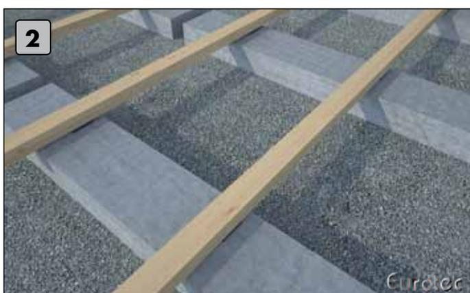
In the versions 1. and 2. a problem becomes clear: You have to work very precisely to bring the top edges of the foundations to exactly the same height. Since this is usually not possible, the supporting joints must be later relined.
