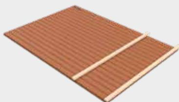
**3** Bolt the lowest rhombus profile to the substructure using the ZK façade screws.
