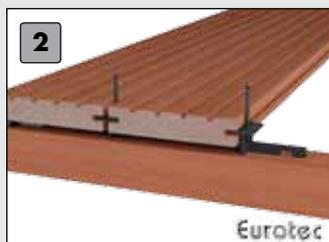
Align and fix the next board, screw down with the T-Stick until all boards are fastened.
