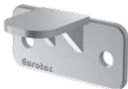
The EVO position anchor provides a simple and straightforward solution for joining Eurotec EVO aluminium system profiles. Thanks to the EVO position anchor, the aluminium profiles can be joined at an angle of between 30° and 90°.
