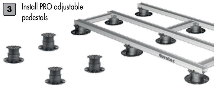
**4** Click EVO aluminium system profile onto adjustable pedestals and extend with EVO aluminium system profile connector so that the entire deck width is covered
