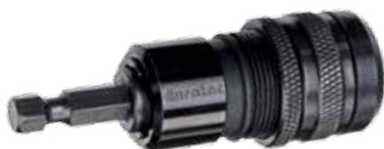
The Screw Stop is the ideal solution for driving screws to an even depth into the wood. In this way, your deck will be given an attractive, even surface pattern. You adjust the required screwing depth with the infinitely adjustable depth stopper. When this is reached, the drive uncouples and the screw stops. You do not have to start again to adjust the seat of the screw head.
