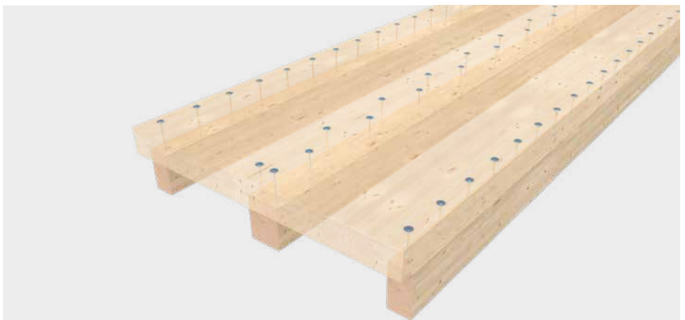
Bonding pressure distribution in the screw press bonding of rib panel elements
