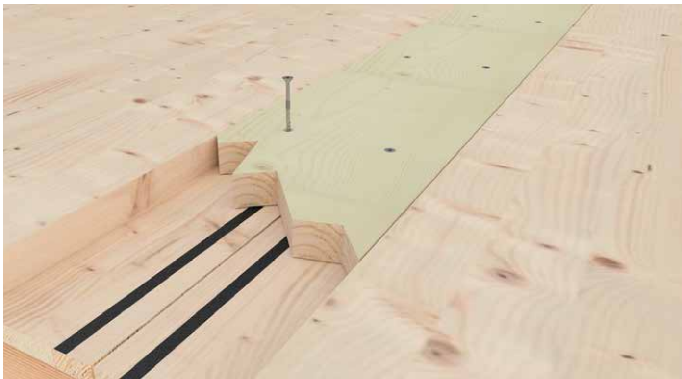
The magazine-fed Panelwistec enables quick and straightforward timber-to-timber screwing through the use of a magazine screwdriver
